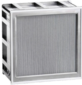
Model: HT350-Pro-H13-610x610x292-01/00 HT350-Pro: Support Flange Type, 350°C H13: Filter Class EN1822 610x610x292: Size WxLxD mm 01/00: Gasket Air Outlet/ Without Grid MGT Ref: HTH3TH3S0KC-610x610x292
